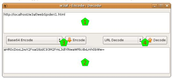
You have two panes where you can insert the text you want; put the text to Encode in the upper pane [1], and when encoded it will appear in the lower pane [2], and viceversa: to decode something put the text in the lower pane and after decoding it will appear in the upper pane.
