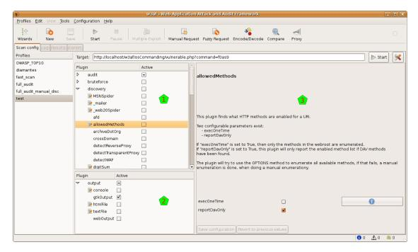
The first section has all the scan plugins, in the upper part of the column [1]. There you have the different plugins grouped regarding the scan type. They are separated in:
