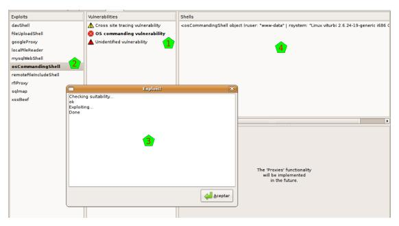
On the other hand, if you actually drag a marked exploit on a marked vulnerability, the system will try to exploit it. A new window will pop up [3], showing the actions that the system is taken. See in the example that the system first checks the suitability of that exploit over that vulnerability, and if OK, it actually triggers the exploit.
