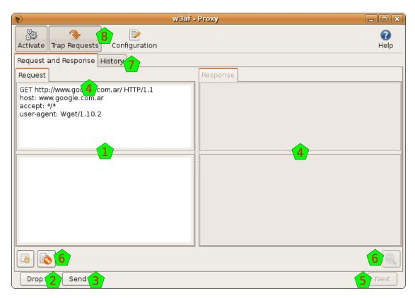
So the system will send the request, and catch the response when arrives, and will show it to you at the right pane [4]. After analyzing the response, you can click on the Next button [5], and the system will pass the response to the other program, and prepare itself to catch the next HTTP request.
