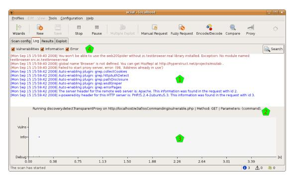
In the lower part of the window you can see a graph that represents what is going on with the scanning process in a visual way. In the x axis you can see the time (automatically rescaled), and in the y axis you can find three indicators: a grey bar which height indicates the quantity of debug messages at that time, a blue dot if there're information messages, and a vertical red bar with the quantity of vulnerabilities found there.
