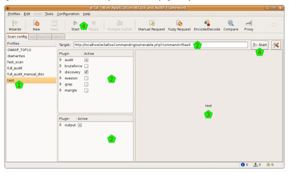
In this example, I selected a test plugin. In the moment I select it, the plugins and the target URL are all reconfigured [2]. Also, in the pane at the right, you can see a description of that plugin [3].
